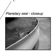
The effectiveness of the planetary seal can be monitored by the simple removal of the planetary motor / gearbox system by removing the four bolts shown below.
