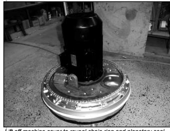
Lift off machine cover to reveal chain ring and planetary seal.
